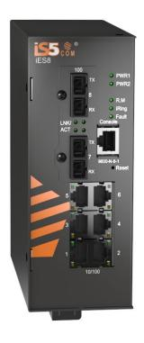
The iES8-S is an intelligent 8 Port managed Ethernet switch with up to 8 x 10/100Base-T(X) RJ45 ports and up to 2 x 100 FX SM/MM SC/ST ports.
