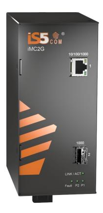
iMC2G is a Gigabit media converter for the conversion of 10/100/1000Base-T(X) RJ45 to 1000Base-X SFP interface which allows extending of communication distance using optical fiber.
