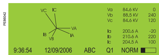
ION8650 front panel phasor display and table.
