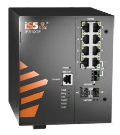
The iES10GF is an intelligent 10 port managed Gigabit Ethernet switch with 7 x 10/100Base-T(X) RJ45 ports, up to 3 x 10/100/1000Base-T(X) RJ45 ports, up to 3 Combo of 10/100/1000Base-T(X) RJ45 and 100/1000Base-X ports, and up to 2 x 100/1000Base-X SFP ports. The switch is IEC61850-3 and IEEE1613 compliant.
