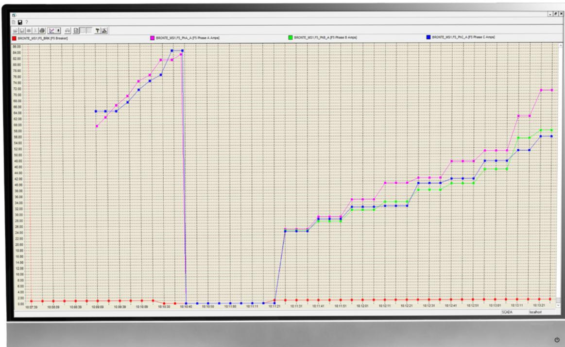
SurvalentONE SCADA displays data collected before and after a disturbance in graphical format. Data is collected using the Disturbance Capture application and shown in the Point Capture Viewer.
