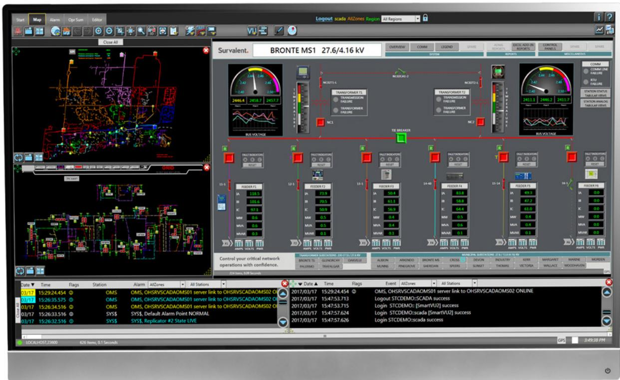
SurvalentONE SCADA can be configured to provide operators with relevant information at a glance. Maps, single line diagrams, schematics, event summaries & alarms are shown in this view.
