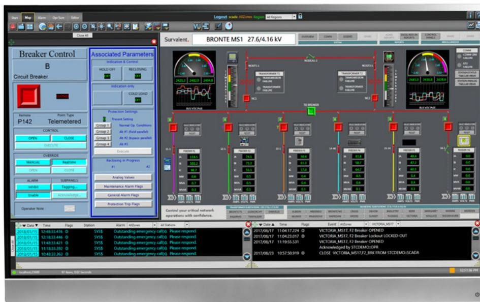
SmartVU allows control room operators to display relevant data in a docked view for easier navigation and faster decision-making.
